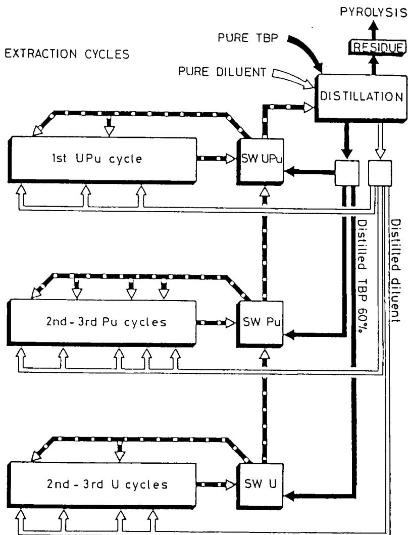
Fig. 1. Solvent management with distillation.
